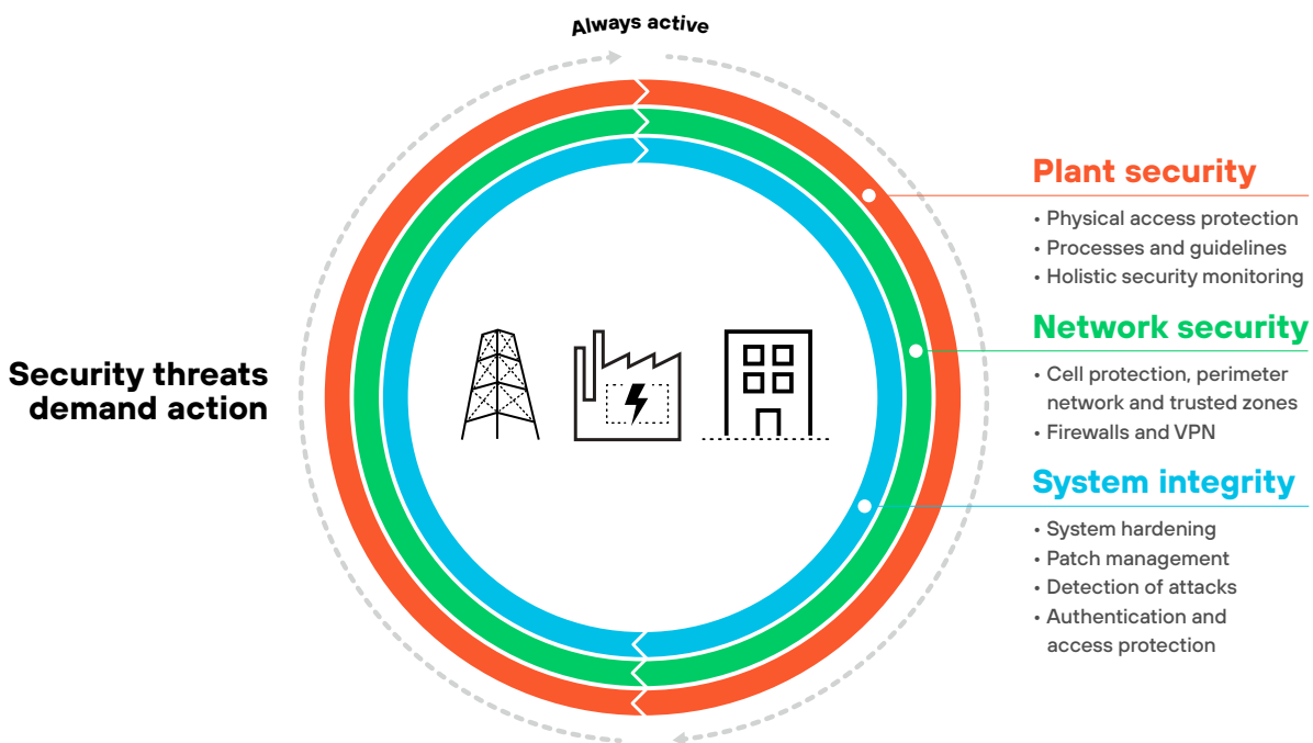
Figure 12: Siemens industrial security concept foundation
